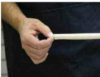
**Step 4.** Carefully wrap the tape around the shaft. Twist or squeeze the end of the tape together, as shown, and push inside the butt end of the shaft. This prevents solvent from entering the shaft during grip installation.
