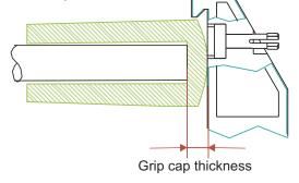
1) Push the grip cap compensator until it clips into position.
