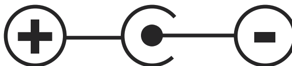
AC/DC adapter and Battery Pack Pin Polarity
