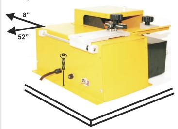
**Step 2:** Familiarize yourself with the shaft clamp/slider assembly. Make sure that the slider is moving smoothly over the guide rods.
