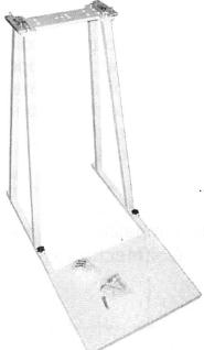
A heavy duty light weight portable bending stand designed to accept both the GolfMechanix & Scotland lie and loft bending machines. This stand features 1"X1" steel box construction, a sliding, reversible standing platform with a treaded steel plate for safety. Backed epoxy finish for durability and attractive looks. Can be bolted to the floor if required.
