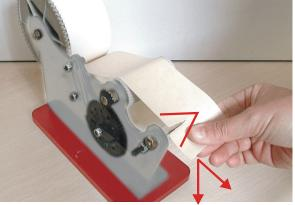
Rip the grip tape over the blade from the inner to the outer edge while pressing down in a swift and deliberate action. The blade holder will automatically collapse, resetting the spools for the next grip tape strip.
