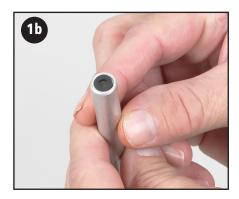
**1.** Insert the replacement washer into the installation tool.
