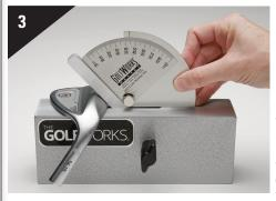
Once the iron head is in place and the sole arm is positioned properly, slide the Golf Club Protractor into position as shown in photo 3, make certain the bottom of the Golf Club Protractor is flush with the gauge surface and the measurement side of the Golf Club Protractor is flush with the sole arm (shown in photo 3). Record the degree reading on the
