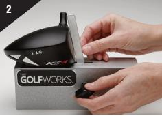
The contact point should be in the center of face (shown in photo 2). The sole arm will usually not contact the entire face surface of the wood due to the vertical roll. Once the sole arm is in place, tighten the knob to prevent the sole arm from moving. It will be necessary to hold the wood head in place with one hand and measure with the other.
