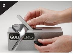
Loosen the sole arm knob to allow placement of the sole arm to the center of the sole. The center of the sole is the intersection of 1/2 the sole width measurement from front to back and 1/2 the sole length measurement from toe to heel. Once the bar is touching the center of the sole, tighten the knob to prevent the sole arm from moving.
