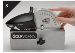
Once the wood head is secure, slide the Golf Club Protractor into position as shown. Be sure the bottom of the protractor is flush with the gauge surface and the measurement side of the Golf Club Protractor is flush with the sole bar (shown in photo 3). Take the reading. The reading will be the loft reading of the club being measured. No calculation is necessary.
