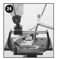
The material of the club head and the experience and preference of the user will dictate which technique is used. To decrease the loft of the putter, pressure should be applied upward on the bending bar. After bending, slide the protractor assembly into position and check the readings to insure the desired loft has been achieved.
