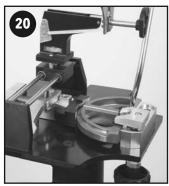
The Maltby Putter Bending machine comes with an adjustable brass bending bar (BNMB). To adjust the lie of a standard style putter (Ping Anser style), place the adjustable brass bending bar on the hosel as shown in photo 22. The bending bar should be parallel to the face. To bend the lie flatter, pressure should be applied downward.
