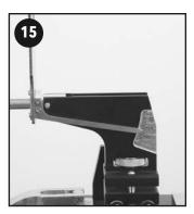
Turn the T-bar bolt until enough space is available to allow the mallet style putter to be placed in the machine. Place the mallet style putter in the machine in the same manner as the standard style putter, with the face flush up against the face block. While holding the putter in position with the face flush against the face block, tighten the T-bar bolt by turning counter clockwise.
