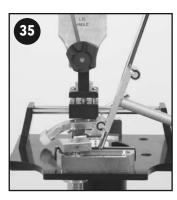
more upright, place the double bend bar parallel to the face of the putter as shown in photo 35. Apply upward pressure to bend the lie to a more upright position. After each time pressure is applied, check the readings with the protractor assembly to see how much the shaft has been bent. Note the position of the head and if it is evident that it has moved from the original, square position, re-adjust and continue the operation. Once the desired lie reading is reached, the operation is complete.
