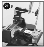
After pressure is applied to bend the lie of the putter flatter or more upright, re-check the position of the face to insure it is still positioned properly in the machine, with the face flush up against face block and the top line of the putter is parallel to the top line of the face block. If any movement has occurred, re-adjust the head into position, and proceed with the bending operation.
