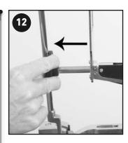
In this instance, the loft reading of the putter is 2°. For left handed putters, install the putter in the same manner as for a right handed putter. Once the putter is in place, simply slide the protractor to the left hand side of the machine, pull the shaft guide into position and read the lie and loft readings in the same manner as the right hand putters (see photo 16).
