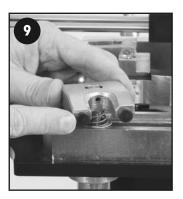
Once the putter head is square in the machine, with the back brace securely tightened, and the top clamp securely tightened (if necessary), the putter is ready for measuring and bending (see photo 11).
