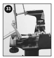
After each time pressure is applied, check the readings with the protractor assembly to see how much the shaft has been bent. Note the position of the head and if it is evident that it has moved from the original square position, re-adjust and continue the operation. Once the desired loft reading is reached, the operation is complete.
