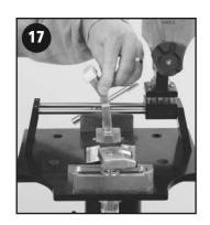
brass knob to raise the shaft guide arm to a position where it can be placed flush on the shaft, above the bend in the shaft. Photo 19 shows a double bend shaft style putter with the shaft guide properly in position to take the lie and loft readings.
