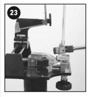
To adjust the loft of a standard style putter (Ping Anser style), the adjustable brass bending bar should be positioned as shown in photo 23. The bending bar should be perpendicular to the face. To add loft, apply pressure downward on the bending bar. A short, quick application of pressure or a constant pressure are the two techniques that are used.
