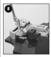
The rubber inserts are designed to prevent marring the top edge of the putter. It may be necessary to snug the top clamp down onto the top edge of the putter to prevent slippage when adjusting the loft and lie of the putter. If it is deemed necessary to use this clamp, position the rubber inserts over the top of the putter and tighten the top clamp by turning the black knob on the bottom side of the machine (see photo 10).
