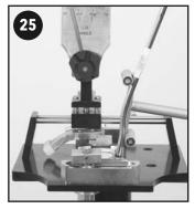
The Maltby Putter Bending Machine also comes with a double bend shaft bending bar (MDBB). To adjust the lie flatter on a putter style that has a double bend shaft, position the double bend shaft bending bar as shown in photo 24. This method positions the lower bending pad exactly at the bend of the shaft. The bending bar should be parallel to the face.
