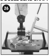
An alternative position of the double bend shaft bar for bending to a flatter lie is shown in photo 25. This places the lower pad of the double bend bar approximately 1" to 2" up the shaft from the head. To adjust the lie flatter, pressure should be applied downward.
