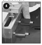
The MA2012 is designed with several key features to aid in installing putters into the machine. Photo 4 shows the two rubber, self adjusting sole pads that helps position the putter square in the machine. The face block (photo 5) is designed with a 4° angle facing the putter face. This angle helps secure the putter head in the machine and prevents slippage when adjusting the lie of a putter.
