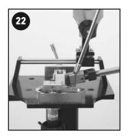
After bending, slide the protractor assembly into position and check the readings to insure the desired lie has been achieved.
