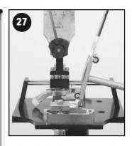
To bend the lie more upright, position the double bend bar as shown in Photo 26. An alternative position of the double bend shaft bar for bending to a more upright lie is shown in photo 27. Note: Either method of positioning the double bend bar can be used on inside the head shaft / head assemblies or shaft over post shaft / head assemblies.
