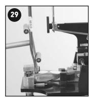
After each time pressure is applied, check the readings with the protractor assembly to see how much the shaft has been bent. Once the desired lie reading is reached, the operation is complete.
