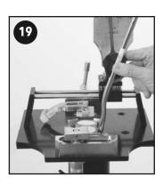
The same procedures used for registering the standard and mallet styles apply for a center shafted putter, with the possible exception of the top clamp application. Depending on the style of the center shafted putter and the length of the blade, the top clamp may need to be positioned toward the toe of the putter. Photos 21A and 21B show a mid size, center shafted mallet properly positioned in the machine, ready for measuring.
