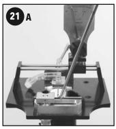
A short, quick application of pressure or a constant pressure are the two techniques that are used. The material of the club head and the experience and preference of the user will dictate which technique is used. To bend the lie more upright, pressure should be applied upward on the bending bar.
