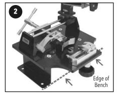
The base of the machine has four countersunk holes that easily line up with the base holes. Four flat head bolts with nuts are included, along with an Allen wrench, for easy installation.
