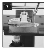
Re-check the position of the putter, making sure the top line of the putter face is parallel to the top line of the face block. The MA2012 also has a top clamp with two round rubber inserts (see photo 9).
