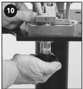
Once the putter is correctly positioned in the machine, position the sliding protractor to the right side of the machine (for a right handed putter). The protractor assembly is designed to give you simultaneous readings of both the loft and lie of a putter. To position the protractor in place for reading, slide the protractor arm forward as seen in photo 12. The sliding arm has a slotted shaft guide that rests up against the shaft for both right and left hand putters.
