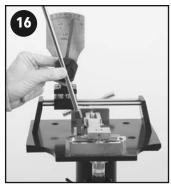
Tighten until the curved back brace is snug up against the back of the putter (see photo 18). If necessary, position the top line bracket as shown in photo 18 and tighten snug by turning the black knob on the under side front of the machine. Photo 18 shows a popular style two ball putter with a double bend shaft correctly registered in the machine. It may be necessary to adjust the height of the protractor arm using brass height control knob (refer to photo 6). If needed, turn the
