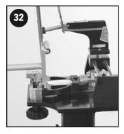
To add loft to a center shafted style putter with the shaft installed inside the head, position the double bend bar perpendicular to the face as shown in photo 32 with the bar perpendicular to the face. Apply downward pressure to increase the loft. To decrease the loft, position the double bend bar as shown in photo 33, again with the bar perpendicular to the face. Apply upward pressure to decrease the loft.
