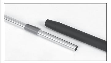
**3.** Abrade the installed shaft from the first mark to the end of the shaft. It is recommended to place a piece of masking tape over the first mark to prevent accidental over abrading.
