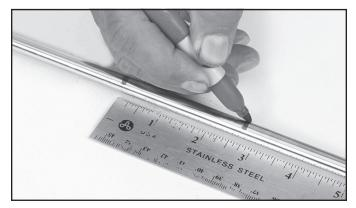
**2.** Place a second mark 2  $3\!\!\!/$  up the shaft. Cut the installed shaft off at this mark.
