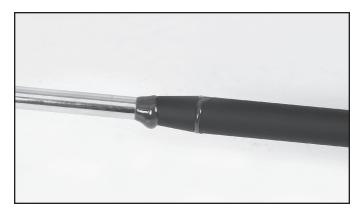
6. Insert the epoxy covered shaft into the aluminum adaptor and Pure Track SS shaft. Work the epoxy covered shaft tip in and out of the Pure Track SS blank and adaptor to ensure proper epoxy coverage.
