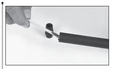
**5.** Apply a generous amount of shafting epoxy to the abraded section of the shaft tip and to the inside of the Pure Track SS putter shaft.
