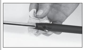
**7.** Using a paper towel dampened with cleaning solvent, clean all excess epoxy from the retro fitted shaft. Let the putter sit in the playing position until the epoxy has dried.
