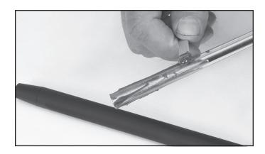
**4.** Apply a generous amount of shafting epoxy to the abraded section of the shaft tip and to the inside of the Pure Track SS putter shaft.
