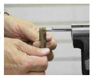
**Step 6.** If you encounter difficulty, use a Ferrule Installation Tool (GW1004) and hammer to start the ferrule onto the shaft.
