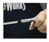
**STEP 14.** After the epoxy has cured, position the club in normal playing position. Slide a 48" Ruler (RUL48) behind the club as shown. Using a felt tip pen, mark the shaft 1/8" below the desired playing length. The grip cap will extend the club's length by 1/8". For steel shafts, use the Golf Shaft Cutter (STC) to cut the shaft at this mark. For graphite shafts, use the Grit Edge Blade (GREB)to cut at this mark.
