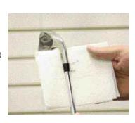
**STEP 10.** Insert the tip of the shaft to the bottom of the hosel, simultaneously rotating the shaft. This will completely coat both the hosel bore and the shaft tip with epoxy.
