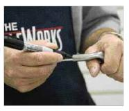
**STEP 5.** If using a ferrule, slide it over the shaft tip. Note: A small amount of epoxy can be applied to the shaft tip prior to installing the ferrule. This helps the ferrule slide into place easier and keeps the ferrule secure.
