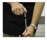
**STEP 9.** Dip the tip of the abraded steel or graphite shaft into the epoxy. Roll the shaft to ensure that the epoxy coats the circumference of the shaft. Take care not to get epoxy on the ferrule.
