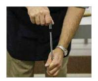
**STEP 11.** Remove the shaft from the hosel. Check to make sure the shaft is evenly and adequately covered. If not, apply more epoxy.
