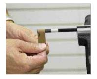
**STEP 1b. Graphite Shaft tip trimming**: Using the Grit Edge Blade (GREB) mounted in a hacksaw frame, cut the shaft per the recommended tip trimming intructions. Apply a piece of masking tape to the shaft at the cutting point to prevent splintering the fibers of the graphite shaft.
